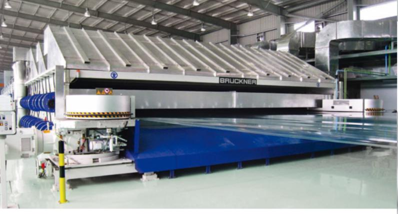
Brückner Maschinenbau is the world's leading supplier of production lines for manufacturing high-quality monoaxially and biaxially stretched films. The lines guarantee efficient, profitable, reliable production of the widest range of flexible films, which are used as high-quality packaging material or for special technical applications, such as capacitors, battery separators or screens and displays.
