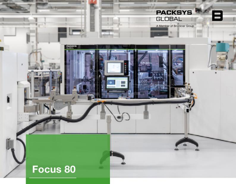
High speed laminate tube line
