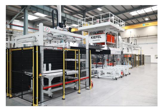
The SHARPFORMER KID 1.250 Smart, a thermoforming machine for high quality inner-liners and door-liners for refrigerators, are produced in Suzhou. © KIEFEL GmbH
