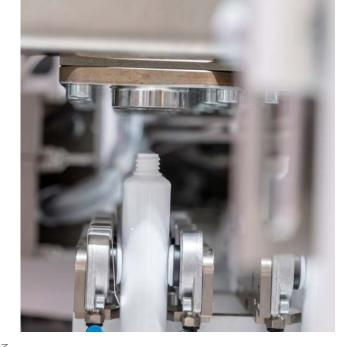
The compression molding header also allows customers to save on storage and handling of injection molded shoulders. The Focus 40 is equip with a high quality tooling which fulfills the requirement of the market.
