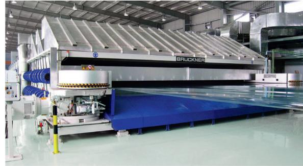
Speed upgrade: the world's fastest BOPP line with 525m/min
